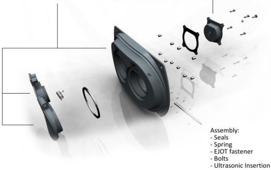
Injection moulding: Polyamide 6 (glassfiber reinforced)
